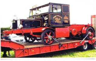
▲ One of only two built, this full restored 100 Tonner's record gross train weight was 165 tons – thanks to a 196-to-1 bottom gear.
