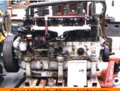
Figure 4 Inlet side of Daimer Knight engine at the Anson Engine Museum
